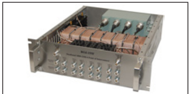
Custom designed RF system for in-building mobile phone applications. Multi-channel combiner/distributor for GSM-900, GSM-1800, 3G and LTE. This product has been widely used for casinos around the world.
