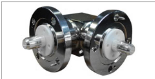
Custom designed EIA 8-13-S adaptor for 10KW UHF TV transmitter. 0-1 GHz/VSWR <1.05/30 Kw peak (Weight 3kg).
