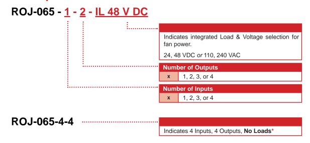
This is a 4 Input / 4 Output Combiner Network – Any unused ports must be terminated.
