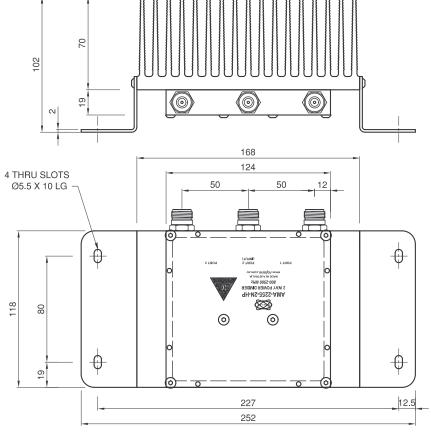
Power Handling – This device has been designed as a power divider. When used as a divider, its power handling capability is 200 Watts maximum input power. If a combiner is required, please see our AMA-072 range of combiners.
