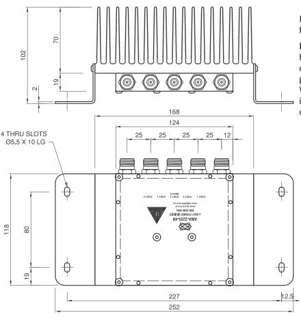
Recommended coupling torque force for N connector 40 to 60 Ncm.
