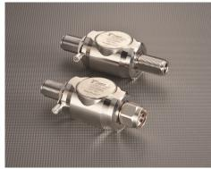
Wireless Broadband applications requiring DC blocking on Center Pin operating from 2000-6000MHz. L1, L2 and L3 GPS protectors with High Pass filter in the RF path and DC pass solid state protection for powering GPS systems
