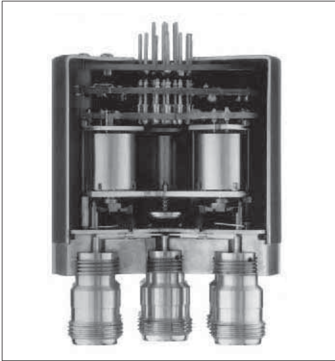
Figure 2: A Cutaway view of RAMSES coaxial switch
