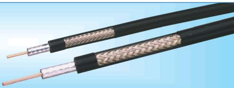
• **Flexible:** With very tight minimum bend radius, LLSB cable can be easily routed into and through tight spaces without kinking. The bonded-tape outer conductor provides superior flexibility and ease of bending compared to previous generation M17/RG type, corrugated copper, or smooth wall copper hard-line cables.
