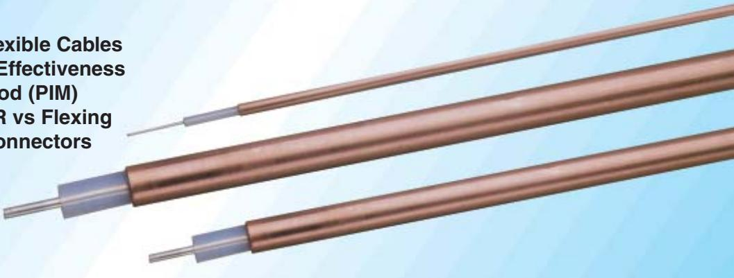
**Coppersol** employs a thin tubular copper outer conductor and solid PTFE dielectric which provides the lowest attenuation and highest shielding giving it significant performance advantages over flexible coax of similar size.
