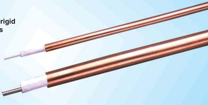
**Coppersol-CLL** employs a thin tubular copper outer conductor and low-density PTFE dielectric which provide the lowest loss and highest shielding giving it significant performance advantages over semirigid coax of similar size.
