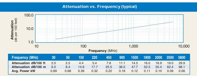
$\begin{array}{l} \textbf{Calculate Attenuation} = (0.356859) \bullet \sqrt{FMHz} + (0.000470) \bullet FMHz \ (interactive calculator available at http://www.timesmicrowave.com/cable_calculators) \\ \textbf{Attenuation: VSWR=1.0; Ambient} = +25^{\circ}C \ (77^{\circ}F) \ \textbf{Power: VSWR=1.0; Ambient} = +40^{\circ}C; \ (nner \ Conductor = 100^{\circ}C \ (212^{\circ}F); \\ Sea \ Level; \ dry \ air; \ atmospheric \ pressure; \ no \ solar \ loading \end{array}$
