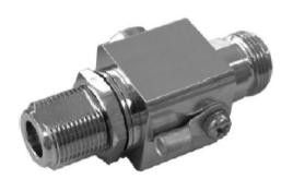
Gas Discharge Tube Protectors contain a gas capsule placed between the inner and outer conductors. Unlike quarter wave protectors, Gas tube surge arresters are broadband devices.
