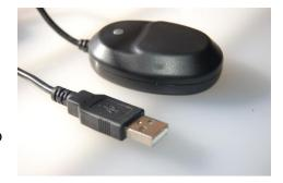
a USB port to allow computer peripherals to be automatically configured as soon as they are physically connected.
