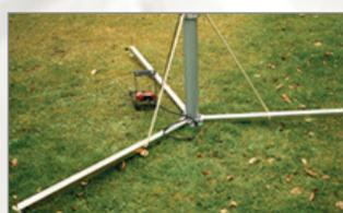
This tripod is designed for the NH Series masts on hard surfaces. It is constructed of steel and folds into a compact unit for storage/transit. It can also be easily detached from the mast. The mast can be rotated and locked in any position and the feet are adjustable to suit uneven ground. The stand is intended for use in light winds only. Top guys are required for windy conditions. **NTRY/89**
