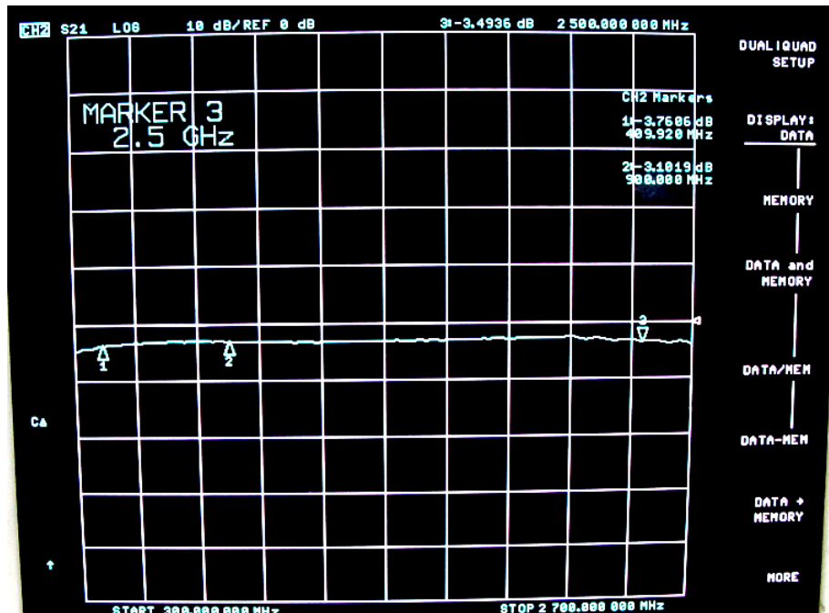
Typical Test Result of 3dB Coupler from 300 to 2700MHz
